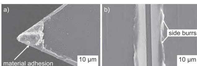
Fig. 19. SEM photographs showing a) material adhesion on diamond tool and b) microgrooves with side burrs. [180].
