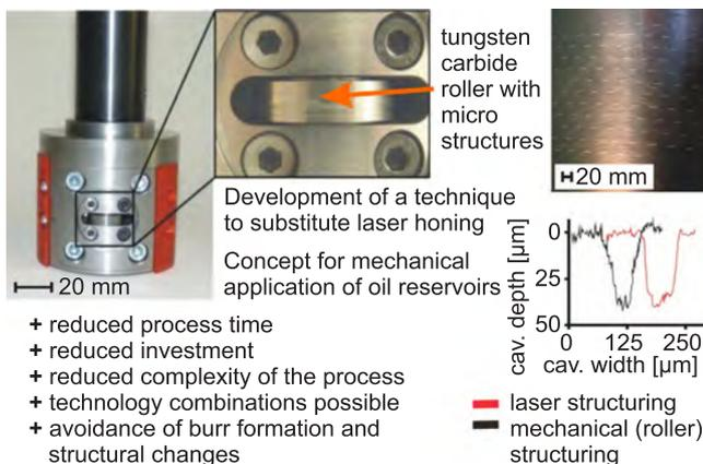
Fig. 27. Micro structuring of cylinder liners by rolling (own work).
