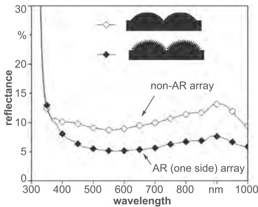
Fig. 7. Reduced reflectance achieved by superimposing nanostructures on microlens arrays. Adapted with permission from [130]. Copyright (2015) American Chemical Society.
