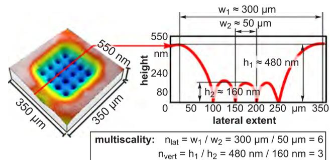
Fig. 2. Exemplary calculation of height and size ratios (calculated for a structure given in [71]).
