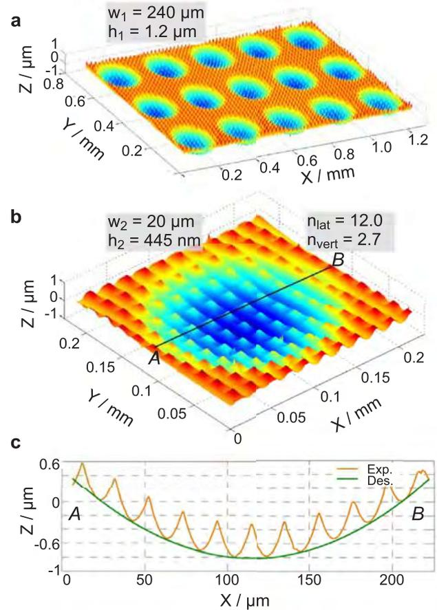
Fig. 13. Characterizations of (a) the microspheric array (MAA) with nano-pyramids; (b) a single microspheric structure with nano-pyramids; and (c) the enlarged view of the secondary nano-pyramids [157].
