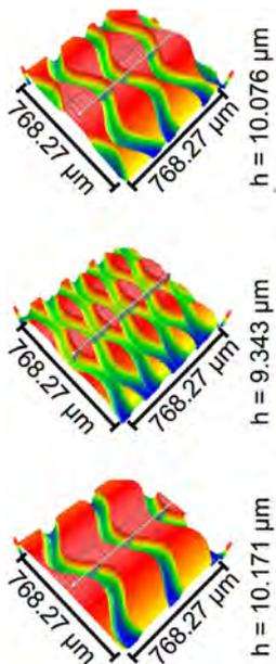
Fig. 15. 3D topography on the roller surface after cutting with varying feed [91].
