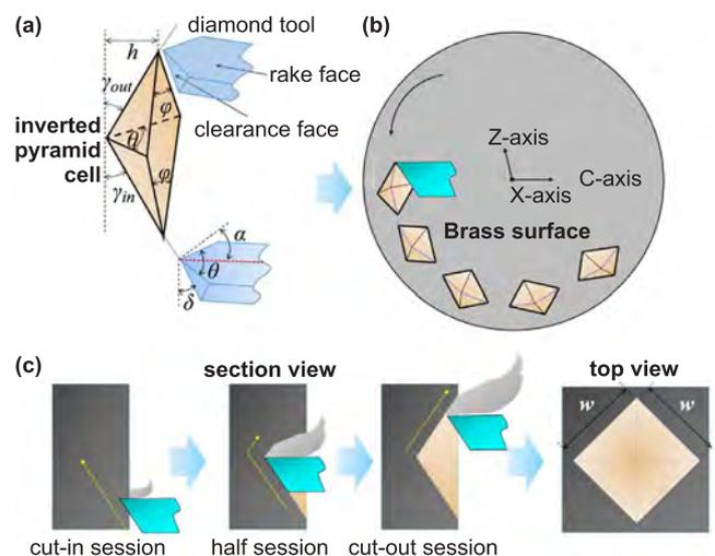
Fig. 21. (a) Geometrical dimensions of engraved cells and the respective cutting tool, (b) Machined inverted pyramid features along the tool trajectory, (c) Motion study of micro engraving in a three-step section view. [74].
