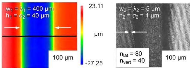
Fig. 4. Multi-scale structured surface for controlled lubricant propagation, adapted with permission from [133].
