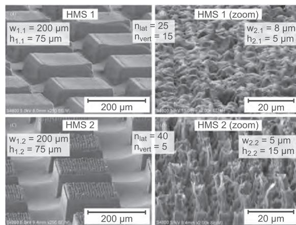
Fig. 28. SEM images of hierarchical multiscale structures on polypropylene surface [77].
