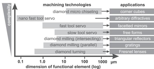
Fig. 45. Selected technologies for generating functional surface structures and related examples, cf. [9,50].
