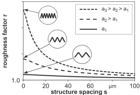
Fig. 11. Dependence of roughness factor  $r$  on structure spacing  $s$  and aspect ratio  $a$  [10].
