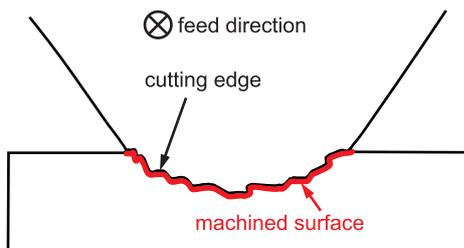
Fig. 12. Secondary surface structuring in fly-cutting by microstructured cutting edges [182].
