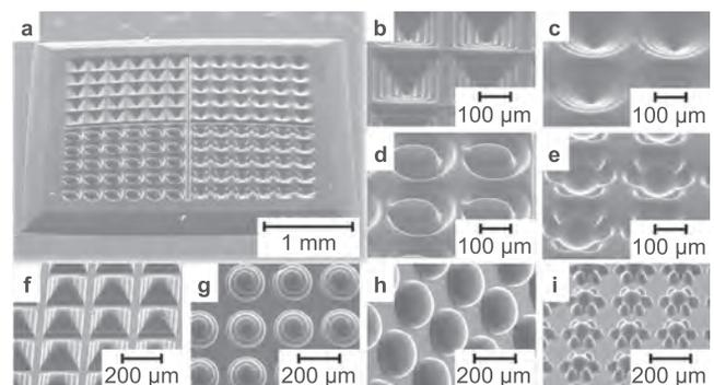
Fig. 44. Microstructures generated by DOPsL [192].
