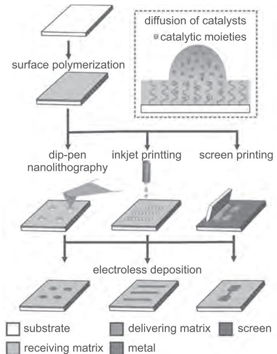
**Fig. 41.** Schematic of matrix-assisted catalytic printing (MACP) process used in dip-pen nanolithography, inkjet printing, and screen printing. [60].
