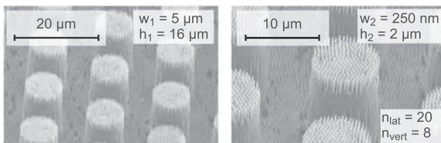
Fig. 37. SEM photographs of hierarchical structures featuring microscale cylinders with nanoscale tips [78].
