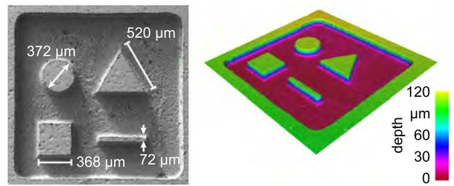
**Fig. 35.** Features machined by dry micro EDM [161].
