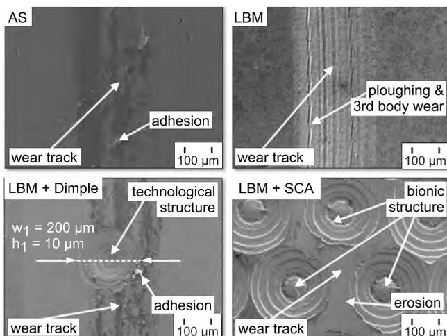
Fig. 5. Wear tracks on as-sprayed (AS), laser machined (LM), technologically (dimple) and bionically structured (SCA) coatings [155].
