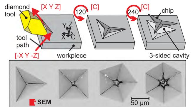
Fig. 20. Diamond Micro Chiseling, process kinematics and achievable structure geometries [10].
