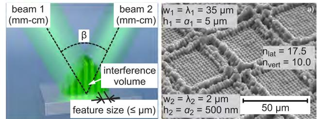
Fig. 31. Schematic for two-beam laser interference patterning [76].
