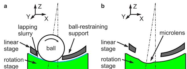
Fig. 25. Schematic of lapping/polishing method for structured mold fabrication, according to [106].
