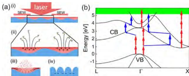
Fig. 30. Schematics of LIPSS formation mechanism on silicon (a) and laser-induced electron excitation (b) [56].
