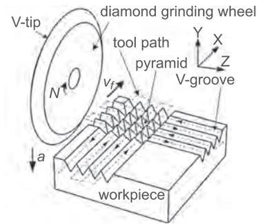
Fig. 24. Grinding for micro pyramid structures [170].
