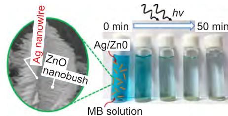
Fig. 8. ZnO nanostructures on Ag nanowires for improved photocatalytic activity [153].
