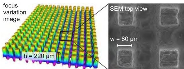
**Fig. 34.** Micro pillars generated by multiple die-sinking EDM [15].
