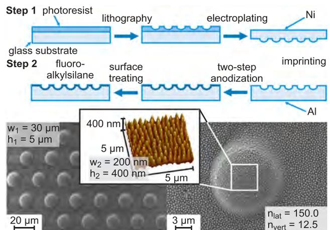
**Fig. 36.** UV nanoimprinting lithography process and multiscale compound eye array [129].
