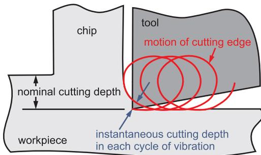
Fig. 18. Elliptical vibration cutting process, according to [151].
