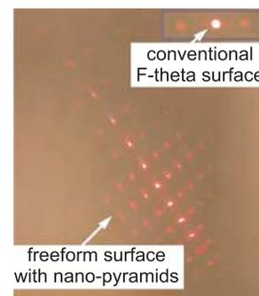
Fig. 14. Reflective diffraction of the freeform surface with nano-pyramids (FFS NP) [216].
