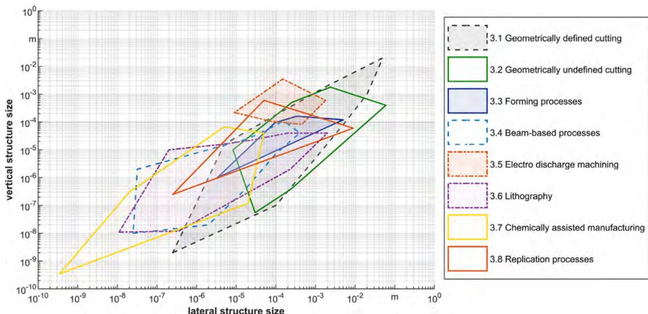
Fig. 46. Size scale of selected manufacturing processes, evaluated from the state of the art.
