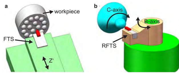
Fig. 16. a) Linear FTS turning of a micro lens structure. b) Rotary FTS turning of a target ball microstructure [213].
