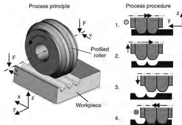
Fig. 29. Principle of incremental rolling for producing defined riblet structures [86].
