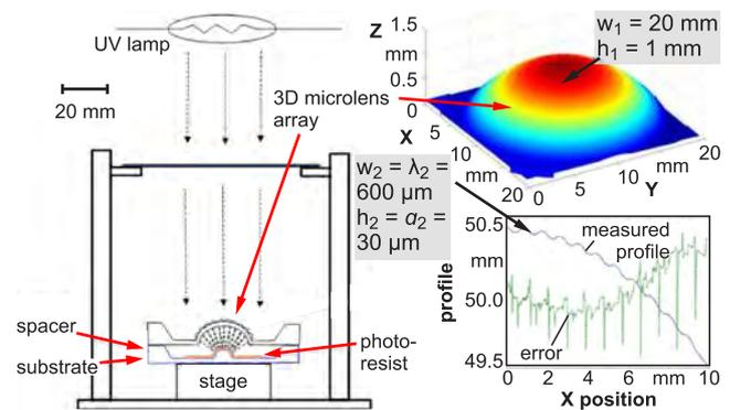
Fig. 6. 3D projection lithography system using a freeform microlens array as developed by Li and Yi, adapted with permission from [100].
