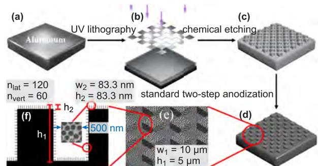
Fig. 39. Ultraviolet lithography followed by two-step anodizing for multiscale structures with super-hydrophilicity [164].
