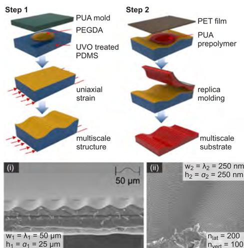
Fig. 42. Multi-step replication of hierarchical structures: fabricating and deforming a structured PDMS sheet (step 1) and replicating a multiscale substrate from this (step 2), adapted with permission from [5].
