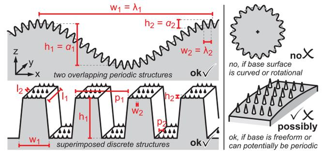
Fig. 1. Characteristic parameters for comparing hierarchical and multiscale structured surfaces.
