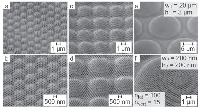
Fig. 43. SEM images of multiscale ommatidial arrays [130].
