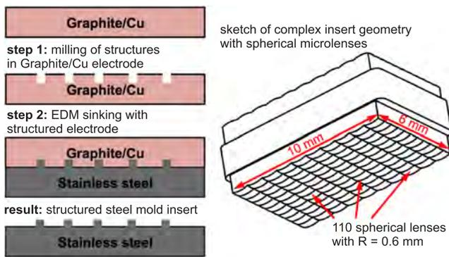
**Fig. 33.** Procedure for hybrid method combining micro milling of structured Graphite/Cu dies and applying these for EDM sinking in steel (left) and geometrical model of lens array (right) [198].
