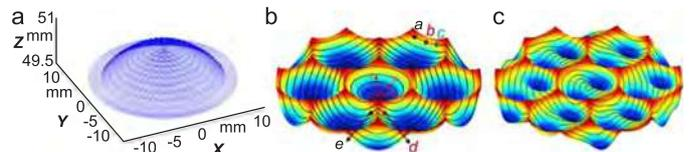
Fig. 17. a) Toolpath of the designed 3D micro lens array for the slow tool servo process [100]. b) Conventional spiral path based fast tool servo diamond cutting of a microsphere lens array and c) a microfreeform lens array [214].
