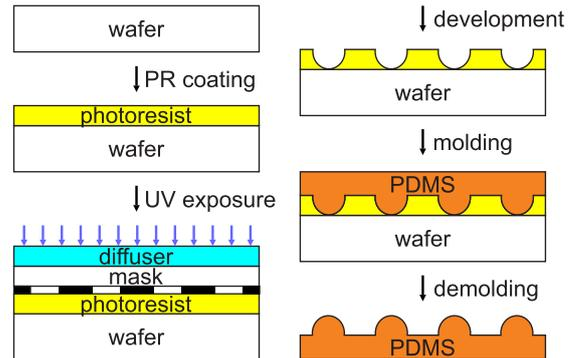
Fig. 38. Combining diffuser photolithography and molding for making microlens arrays, according to [80].
