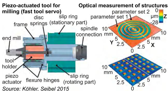
Fig. 9. Micro structure generation with a fast tool servo in milling, cf. [89].
