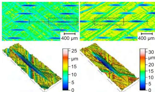
Fig. 26. Cylinder surface with prismatic inserts by honing [25].
