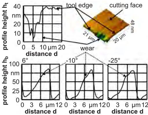
Fig. 22. Wear profile of the tool edge (top), effect on the nanostructure (blazed grating) dependent of the sagittal slope (bottom). [159].
