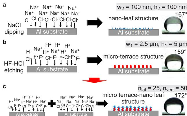
**Fig. 40.** Schematic illustration of formation of (a) nano-leaves by dipping in NaCl solution, (b) micro-terraces by etching in Beck's etchant, and (c) microterrace nanoleaf hierarchical structures by etching and subsequent dipping in NaCl solution [85].
