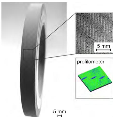
Fig. 23. A surface-patterned grinding wheel [27].
