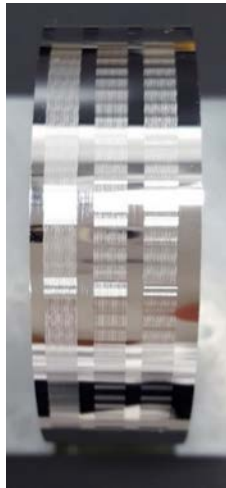
Fig. 17. Photograph of a roll mold of aluminum alloy.
