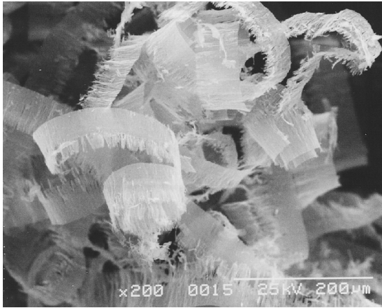
Fig. 4. SEM photograph of ribbon-type chips of silicon generated at an undeformed chip thickness of 58 nm.
