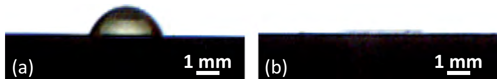
Fig. 15 Photograph showing water droplet on (a) original surface (b) after cone generation
