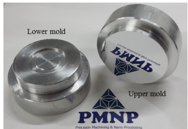
Fig. 4. Photographs of fabricated aluminium molds.
